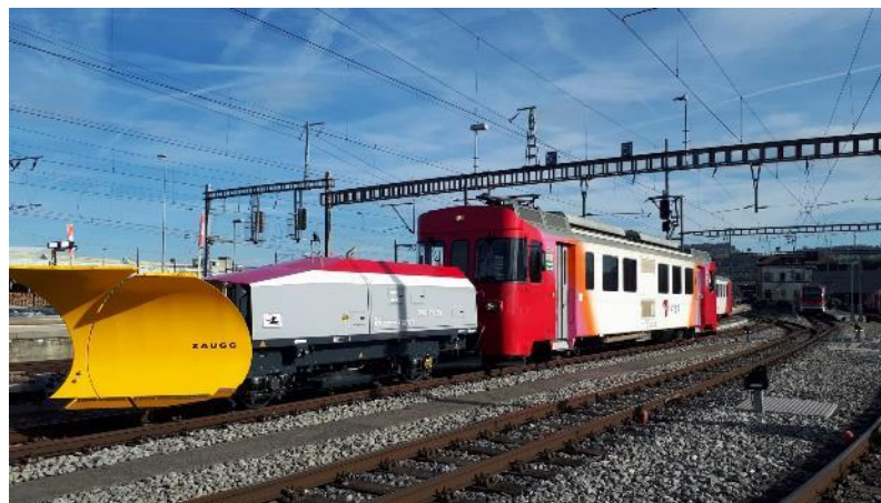
Wagon-lame Zaugg (2022) type NStCM + Fraiseuse
